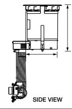
HWB-4QT (4-Liter)Series 9.67" (246 mm) HWB-7QT (7-Liter) Series 8.61" (219 mm) HWB-11QT (10-Liter)Series 8.71" (221 mm)
