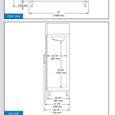
**IMPORTANT NOTE:** If the cabinet is located directly against a wall and/or under a low ceiling, a <u>minimum</u> clearance of 12" is required on top and 3" on sides and rear.
