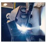
Robotic welding is precise, virtually eliminating leaks.
